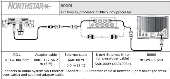
Max Ethernet cable length from RI11 box to switch/display is 50 m.
