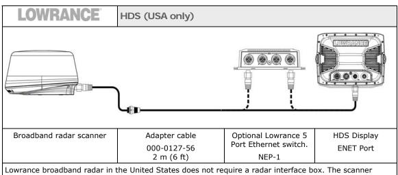
Lowrance broadband radar in the United States does not require a radar interface box. The scanner connects directly the display or Ethernet switch via the adapter cable.
