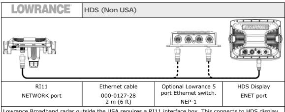
Lowrance Broadband radar outside the USA requires a RI11 interface box. This connects to HDS display via Ethernet either directly into the ENET port on the display or by using an optional 5 port Ethernet switch. An additional Ethernet cable will be required.
