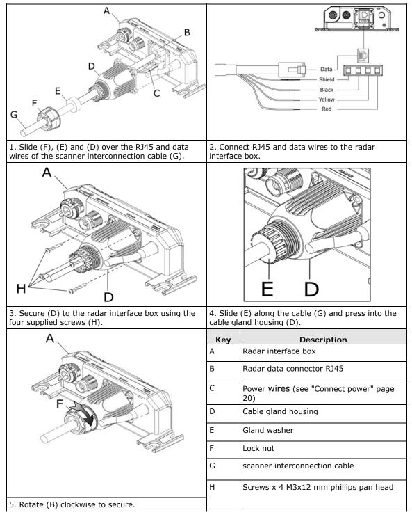
To remove the scanner interconnection cable follow the above procedure in reverse R order.
