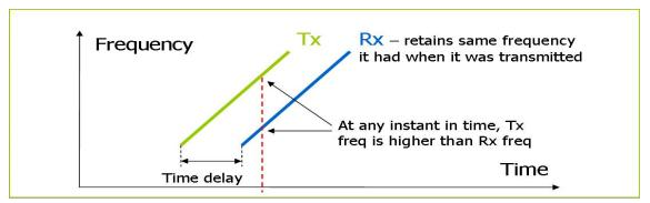
The difference between both the currently transmitted and received frequencies, coupled with the known rate of frequency increase, allows a time of flight to be calculated, from which distance is calculated.
